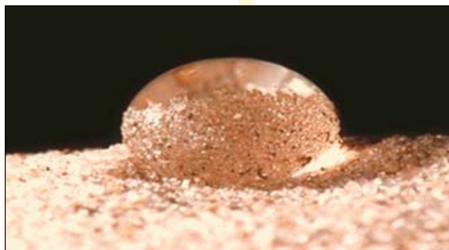
Figure 2: Water droplet on surface of non-wetting soil.
